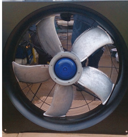
Figure 1: The aerodynamic EC fan has aerofoil-shaped swept blades with winglets, and a serrated trailing edge
